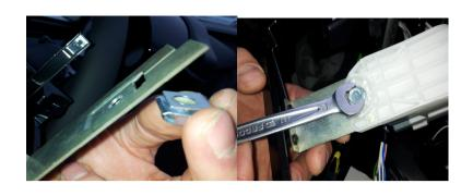
FASTEN THE PLASTIC HOLDER ON THE METAL PLATE SUPPLIED USING THE OEM SCREW AND CLIP
